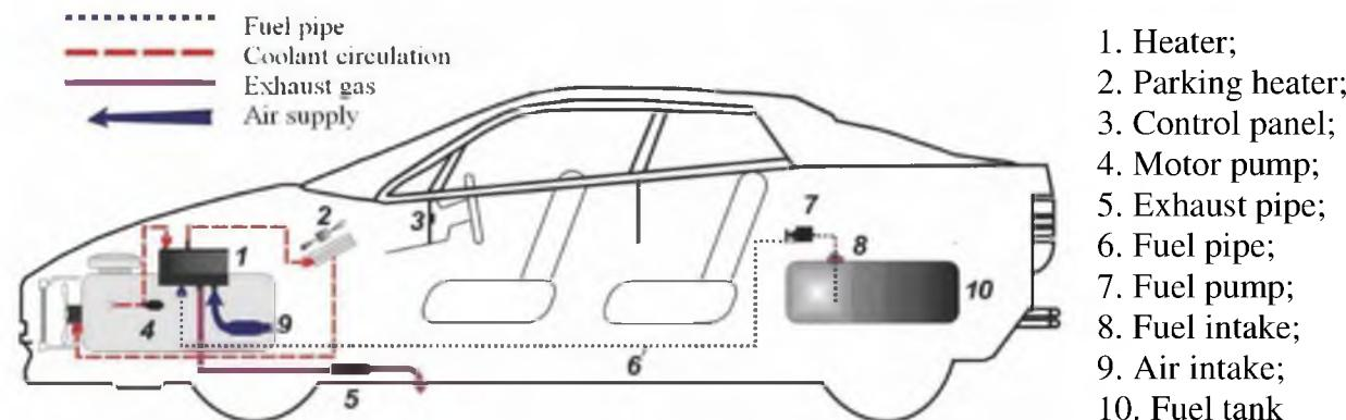
Figure 7.1 - Pre-heater installation diagram
