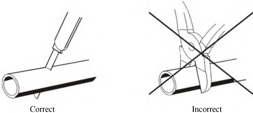
Figure 7.9 – Cutting the fuel pipe before installation
