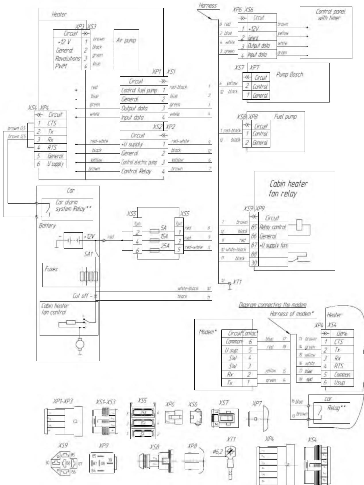
\* Installation of the modem with special harness (with additional orders), which are installed instead of the harness going to the alarm relay.
