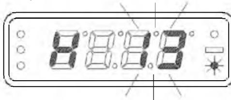
Figure 6.24- indicator shows the pre-heater fault.
