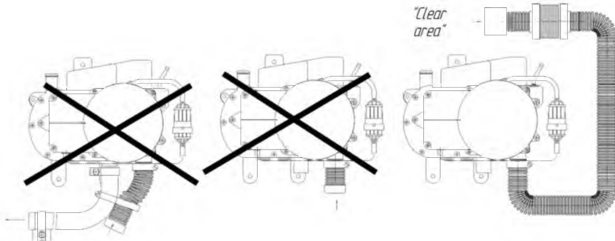
Figure 7.3 – Installation of the air intake
