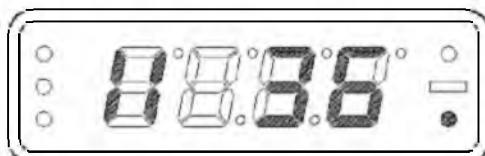
Figure 6.16 Cooling-down mode
